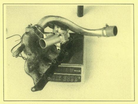
The intake manifold fitted on the car is fitted with a red pipe (see above photo). On the homologation form A5743, the intake manifold is shown with a blue pipe. This red pipe is not complying with homologation form A5743.
